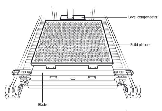
Figure 6: Upper printer compartment view (open)
