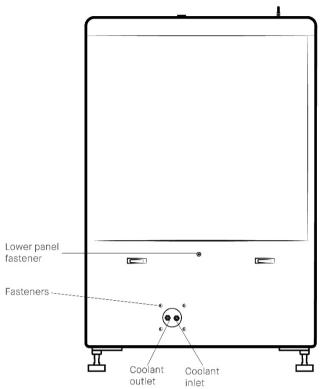
Figure 5. Left-side view of the printer
