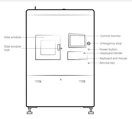
Figure 4. Right-side view of the printer
