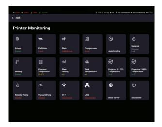
When print job starts, the system detects the required temperatures for the chamber, blade, and material tank and heats the components to the minimum required temperatures indicated in the job file. There is an option to abort the job during the printing process.
