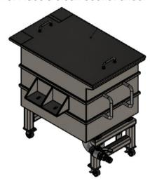
Figure 13: Material Tank and Drain Valve
