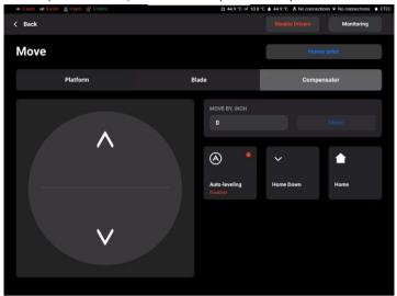
Set the value of one step in the **Move By** field using the keyboard. Press **Move** to move the compensator for the indicated distance towards one of the following directions:
